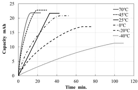
Charge : CV / 2.7V / cutoff 0.2C / -40°C, -20°C, 0°C, 25°C, 45°C, 70°C
