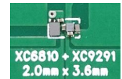
Multi-function charging IC Achieves ultra-compact size together with a step-down DC/DC.
